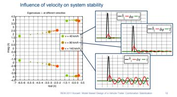
Investigation on the influence of different parameters on system stability Eigenvalues  $\lambda$  of systems with different masses dψ/dt m m Frag = 2000 kg m Hath = 500 kg  $-\gamma$ 🔴 m <sub>Fra</sub> = 1750 kg m<sub>bob</sub> = 750 kg Investigation on influence of different parameters: Mass and mass of inertia of vehicle, distance between the axles of vehicle, distance between trailer coupling and rear axle, mass and
