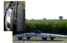
Q™ axial flux PM motor used in American Solar Challenge by the North Dakota State University (Source: Bodine Electric Company)
