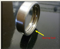
Outer race fault
