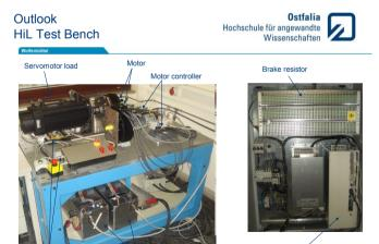
Vehical controller sensor simulation
