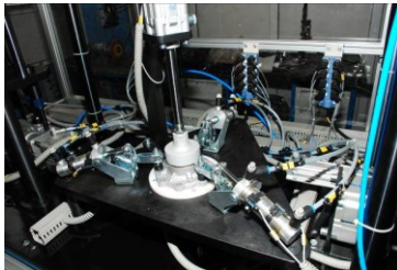
Figure 4 control station for "coupling" PTU
