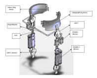
Fig.3. Functional model, constructive component
