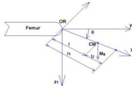
Fig.8.The calculation of the reactions in the joint.
